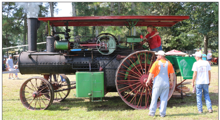
This FRICK steam tractor, built in 1915, was on the grounds at Piney Chapel, with a full head of steam built up to run its belt-pulley as a power source for a wheat thresher demonstration.
