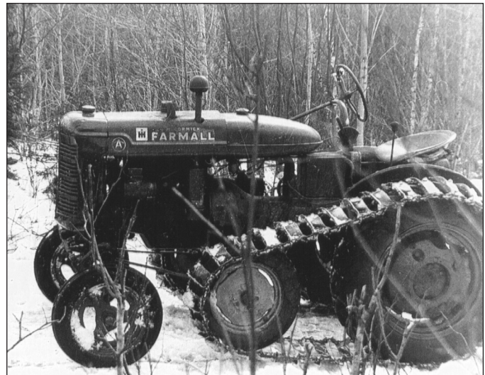
This is how the '47 "A" looked with the "half-track" system installed. The improved traction it provided made a big difference in heavy snow.
