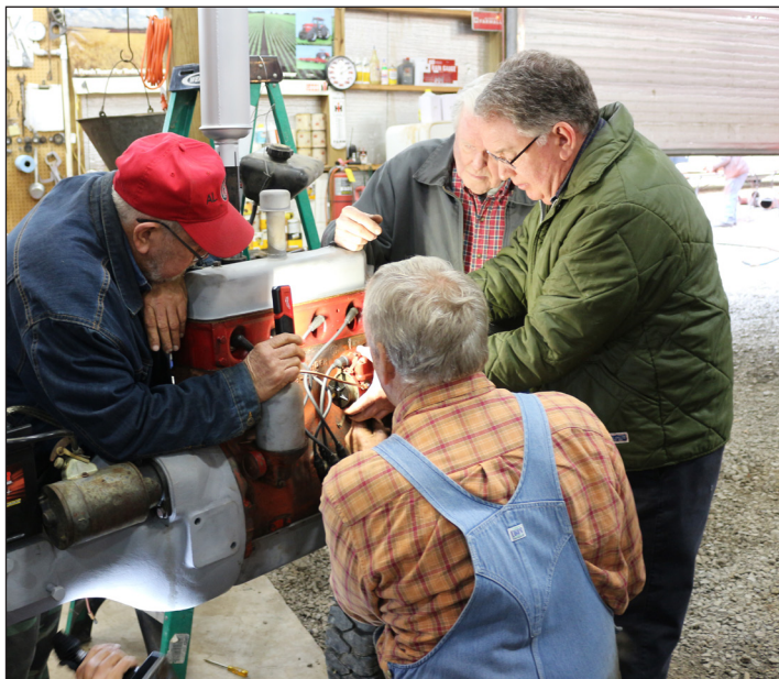
(Left) It took some good teamwork to get the magneto set and timed correctly. (Above) Leonard Summerford climbed into the cotton basket to hammer out dents in the steel mesh while Larry Lemmond held a small anvil for him.
