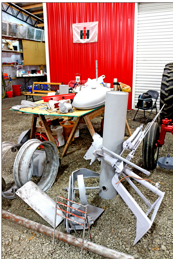
(Left) Sanded and primed parts wait for reassembly to begin. (Above, L-R) Glen Sanders, Sherman Roberts, Robert Bodine, Buddy Banks and Gary Bell reinstall the motor after a complete clean-up and rebuild.
