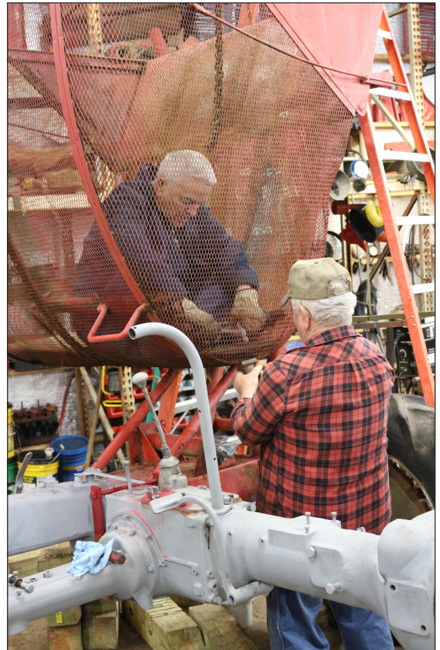
(Left) It took some good teamwork to get the magneto set and timed correctly. (Above) Leonard Summerford climbed into the cotton basket to hammer out dents in the steel mesh while Larry Lemmond held a small anvil for him.
