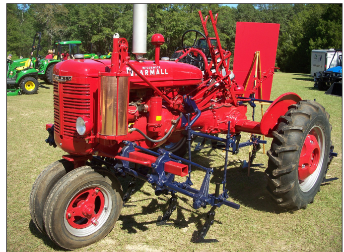
A nice Farmall B restoration with cultivators and rare exhaust lift as seen at the show at Dothan in October.
