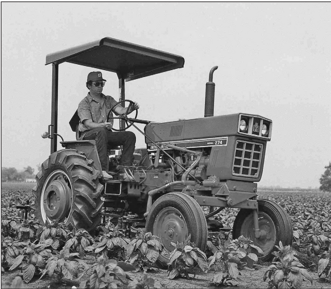
The Japanese manufactured IH 274 offset tractor. Photo from International Harvester Tractors, 1955-1985 by Ken Updike, page 120.
