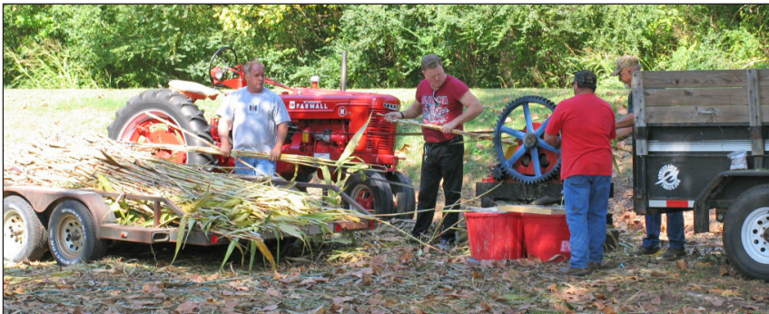
Tim Brasher of Shelby, AL (#277), next to trailer, helps feed sorghum cane into the crusher at the Shelby Ironworks Fall Festival in October, 2012. Tim used his Farmall H for belt pulley power to the mill. The juice was then cooked into syrup.
