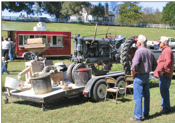
Tim Brasher of Shelby, AL (#277), next to trailer, helps feed sorghum cane into the crusher at the Shelby Ironworks Fall Festival in October, 2012. Tim used his Farmall H for belt pulley power to the mill. The juice was then cooked into syrup.
