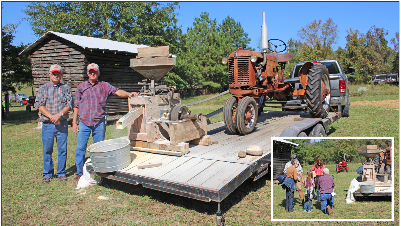
Joe Criswell (#357) and his friend Larry Aldredge with Larry's original condition Meadows belt powered grist mill. You'll see Larry and Joe demonstrate old-time corn grinding at shows through out the season. Kids love seeing how grits, cornmeal, and chicken feed used to be made. Until recently, they used a hand-crank Farmall F-12 for power. At Peinhardt, they brought an electric start CASE tractor to make the work a little easier.
