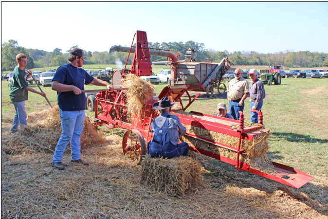
Baling hay at Peinhardt using a stationary engine powered baler. The seated men are tying each bale by hand with wire.
