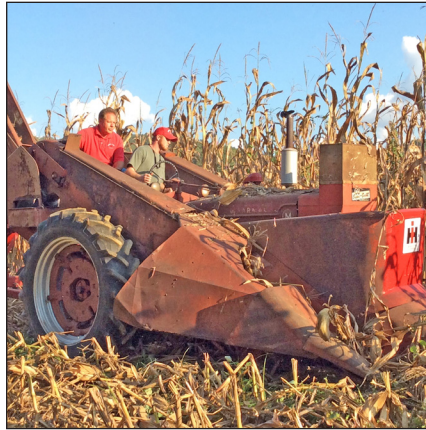
Robert Bodine (#170) watches Matt Bodine (#311) take a turn running Robert's latest project – a 234 IH two row corn picker mounted on an M Farmall.
