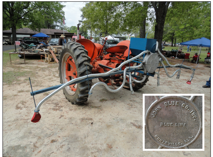
A John Blue cotton duster attached to a tractor at Houston, MS. The apparatus was manufactured in Huntsville, Alabama.
