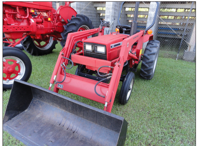
This IH model 244 was part of IH's effort to break into the "small tractor" market in the early 1980's. This tractor has 18 hp and a 3 cylinder diesel engine. IH partnered with the Mitsubishi company in Japan for the model 254, 244, and 234.
