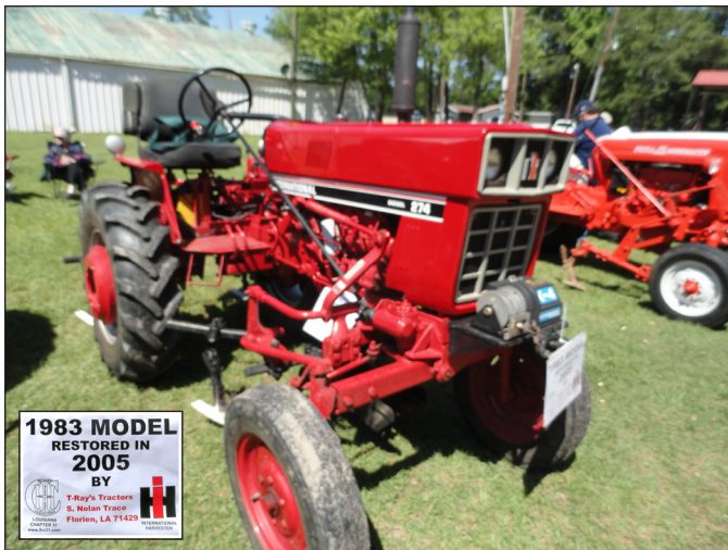
This rare IH model 274 diesel was on display at the Louisiana show. This tractor was International's last effort at an "offset" tractor and replaced the "Cultivision" model 140. They were manufactured and imported from Japan.
