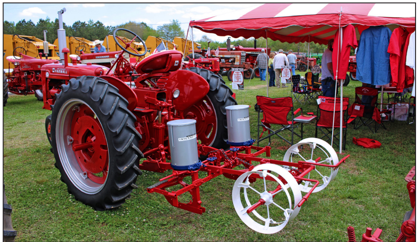
(Right) Robert Bodine (#170) with Bodine Farms brought to Snead this good looking Farmall Super C with a perfectly restored two-row, two-point fast-hitch C-251 McCormick International Planter attached.
