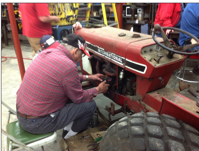
Ray Best (#97) removes a carburetor from an International 184 Cub Lo-Boy At the Bogalusa, LA Cub Fest in March. Cubs needing repair get the attention of the experts at this event.
