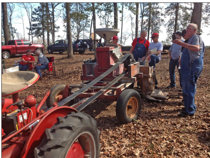
Buddy Banks (#228) demonstrates grinding corn meal using an IH mill powered by a Cub belt pulley at the Deep South Cub Fest in Sneads, FL in early April.
