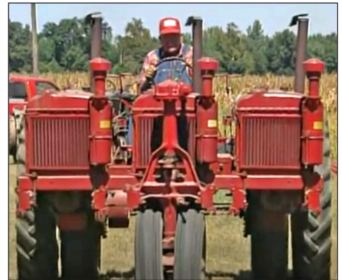
Harry Lee at the wheel of his triple F-20, just one of several tractors he designed and built powered by more than one tractor engine and drive train.
