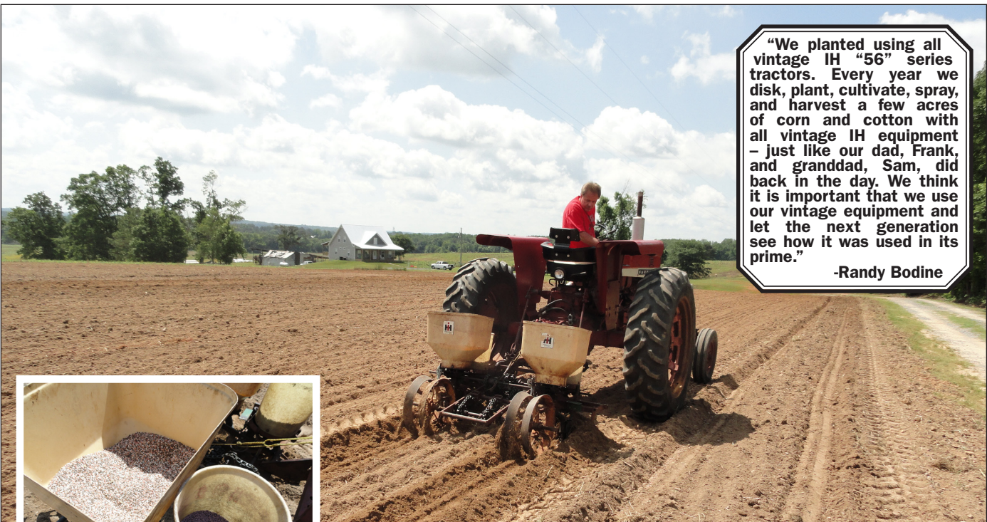
Robert Bodine (#170) operates a two row IH planter mounted on a Farmall 656 Diesel. The photo at left shows the hoppers that hold fertilizer and seed for the planter to distribute. The planter unit plows two rows at a time, drops the fertilizer and seed at the proper interval, and then packs each row, all in a single pass.
