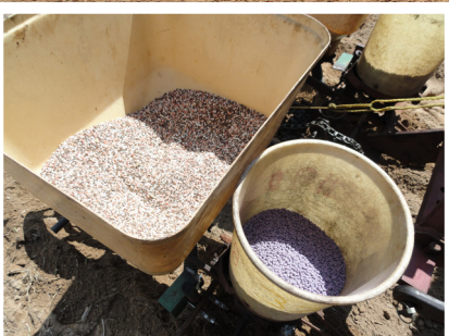
Robert Bodine (#170) operates a two row IH planter mounted on a Farmall 656 Diesel. The photo at left shows the hoppers that hold fertilizer and seed for the planter to distribute. The planter unit plows two rows at a time, drops the fertilizer and seed at the proper interval, and then packs each row, all in a single pass.
